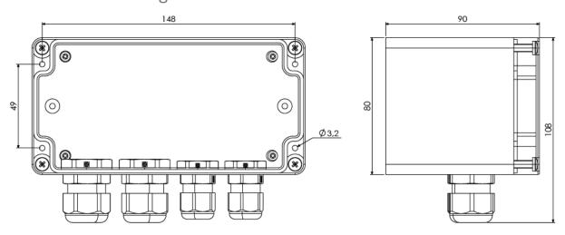
The enclosure is assembled using the four 3.2 mm diameter holes. OBSTA recommends using M3 screws with lock nuts.
