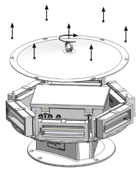
To access the OFI-360 internal cabinet, unscrew the six nuts using an 8 wrench. Rotate and lift the cover. Open the case to access the PCBs.
