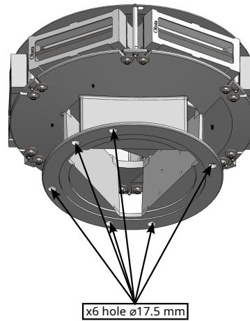
The OFI-360 is mounted through the six 17.5 diameter holes on the beacon base.
