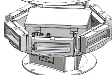
To access the OFI-360 internal box, unscrew the six M5 brake nuts using an 8 wrench. Rotate and lift the cover. Open the case to access the PCBs.
