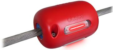
The power supply by inductive effect ensures a light intensity compliant with ICAO red fixed low intensity with infrared when the value of the electric current crossing the line is by default above 20A, whatever is the voltage of the power line
