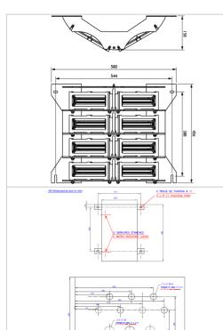
High intensity flash-head consisting of 8 projectors coming with 3 meters of molded cable and a stainless bracket
