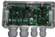
**Monitoring box allowing the control and the wiring of 1 to 4 NAVILITE 48VDC beacons, operating at night only or continuously, plugged to work simultaneously or 2 in redundancy (a main light and a backup light working only in case the main light is not working) with remote signalization in case of failure of the light or failure of the 48VDC supply**
